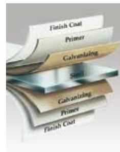
Steel skins are protected through a tough, layered coating system, including a hot-dipped galvanized layer, a protective metal oxide pretreatment and a baked-on primer and top coat.
