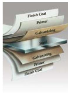
Steel skins are protected through a tough, layered coating system, including a hot-dipped galvanized layer, a protective metal oxide pretreatment and a baked-on primer and top coat.
